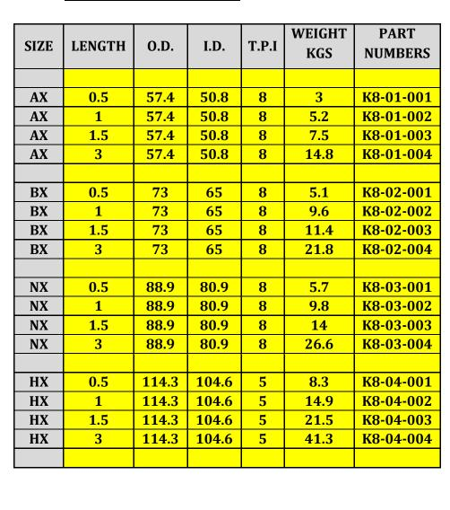
ALL KUVAWALA CASINGS ARE MANUFACTURED FROM THE HIGHEST QUALITY RAW MATERIALS i.e. COLD DRAWN SEAMLESS TUBES OF GRADE SAE 1541 THAT ARE IMPORTED. THESE HAVE EXTREMELY HIGH MECHANICAL PROPERTIES AND STRAIGHTNESS BETTER THAN 1:2000. ALL DRILL CASINGS ARE PARALLEL WALL
